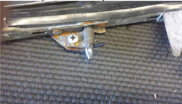
**17** Install travel limiting roll pin and tension screw, insure glass is properly aligned and functions properly; many adjustments may not be made after assembly is installed in the door.
