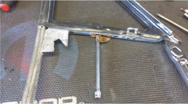
**11** Adjustments to the angle of the glass can be made front to back or in and outward using a 1/4" extension as shown
