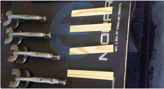
**1** Tools required clamping vent frame to vent post vise grips and paint sticks
