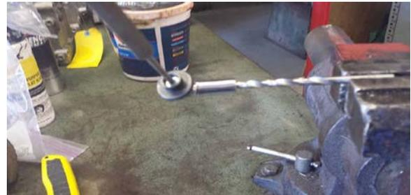
**14** check pivots fit to pin if pivot does not slide completely onto pin then it will need to be deburred this can be done as shown with a small drift for leverage and a 3/16" drill clamped in a vise, several rotations may be required.
