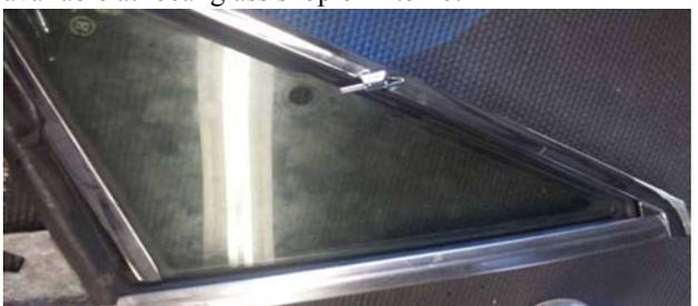
**10** Install vent glass assembly in frame to check for necessary adjustments to center glass and proper seal to gasket follow steps 11 and 12 to adjust
