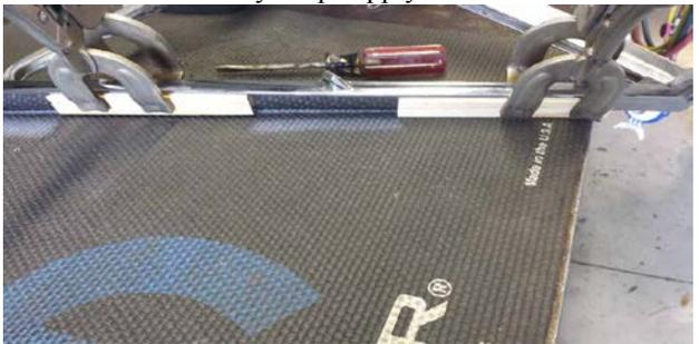
**6** Clamp frame to post at each end, be sure not to clamp on top of alignment pins, allow to adhesive cure over night
