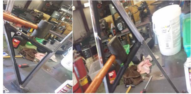
**12** Adjustments up and down can be made by properly supporting frame assembly as shown on a hard rubber pad or block of wood to prevent scratching and then striking with rubber mallet.
