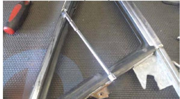
**16** If adjustment needs to be made to pin alignment it can be done as shown with 1/4" deep socket and extension.
