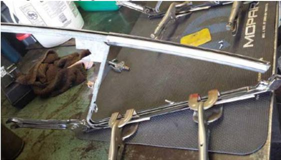
**3** Trial fit to adjust vise grips as show using paint sticks to protect chrome
