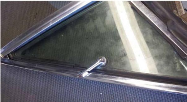
**15** Install pivot to glass assembly (do not tighten pivot screw) lock vent window and insure glass remains in proper position and then tighten pivot screw. Note: in some cases pin may need to be adjusted, see next step
