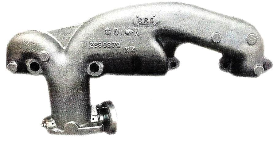
everything with a high horse engine in it. Correct from the factory part numbers, casting ID marks, and casting dates, these are identical copies of the long-gone originals and probably one of the most universally needed parts introduced last year. Licensed by Chrysler as an authentic repro part, these big beauties are absolutely perfect. For more info, contact Tony's Parts, at 302-398-0821.
